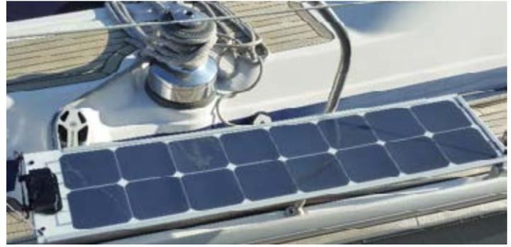
When the sun is directly overhead, the rays are the most direct and intense. As the sun becomes lower in the sky, the same area of light covers a larger area of earth, the intensity decreases and the solar panel output decreases.
